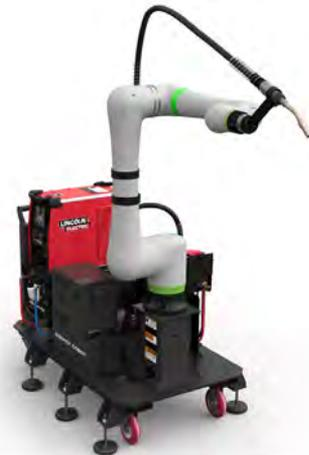
Cooper CRX-25iA Air-Cooled Wire-Break Welding Cobot Cart
