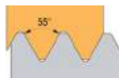
Rosca Interna Perfil Total Full Profile Internal Thread Filetage Intérieur Profil total
