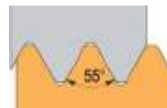
Rosca Interna Perfil Total Full Profile Internal Thread Filetage Intérieur Profil total
