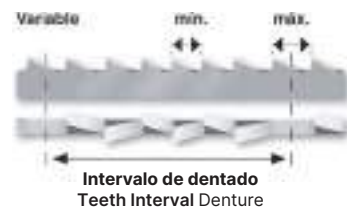
Dentado variable Variable tooth pitch Denture variable
